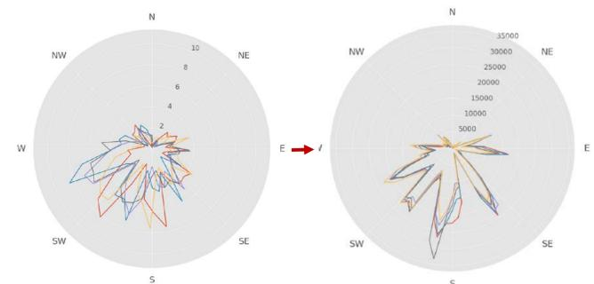
**Directional curtailment:** Depending on the direction in which the curtailment occurs, a shift in direction can generate non-negligible production losses. For the wind farm considered in the study, a shift of 30° results in a net loss of 13 000€ and non-compliance with regulation
